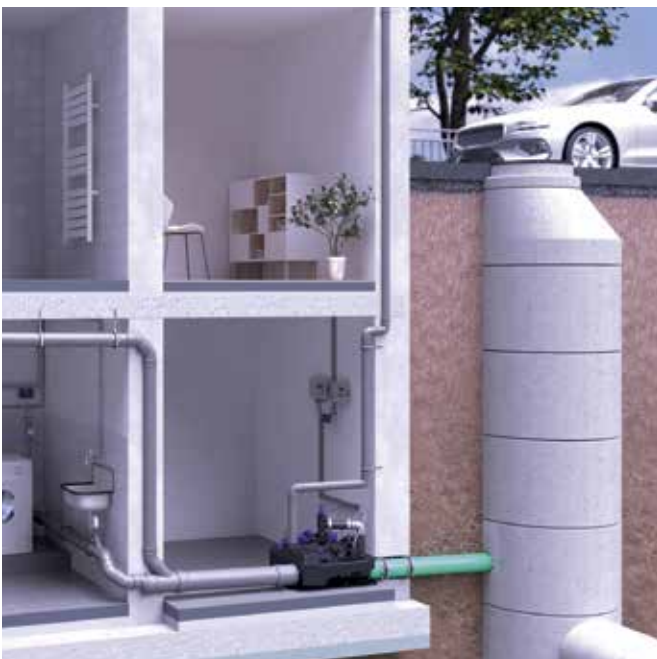
Ecolift L Bypass (FKA) on the ground floor of an apartment building below the backwater level
